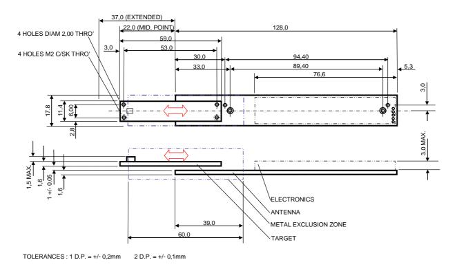
Recommended installation method is to align the unit using M2 plastic dowels then secure with adhesive (such as 2 part epoxy) and/or nylon M2 screws.
