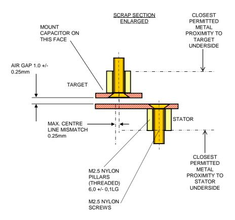
Note – air gap should be maintained within limits to ensure stated maximum non-linearity. Air gaps outside this tolerance will increase non-linearity. Generally – up to a limit – non-linearity will increase by +100% for each 100% increase in tolerance band. Resolution and repeatability are generally independent of air-gap up to a tolerance of +/-1.0mm from nominal.
